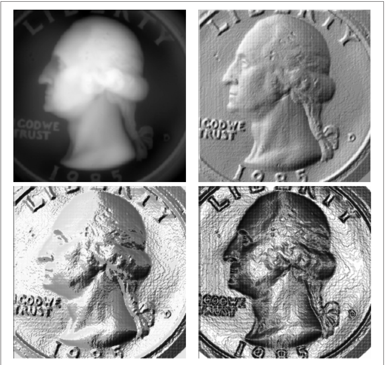
Figure 50. Range image of a coin (produced by a scanned stylus microscope), and three renderings using Phong shading with different specularity and incident light positions.
