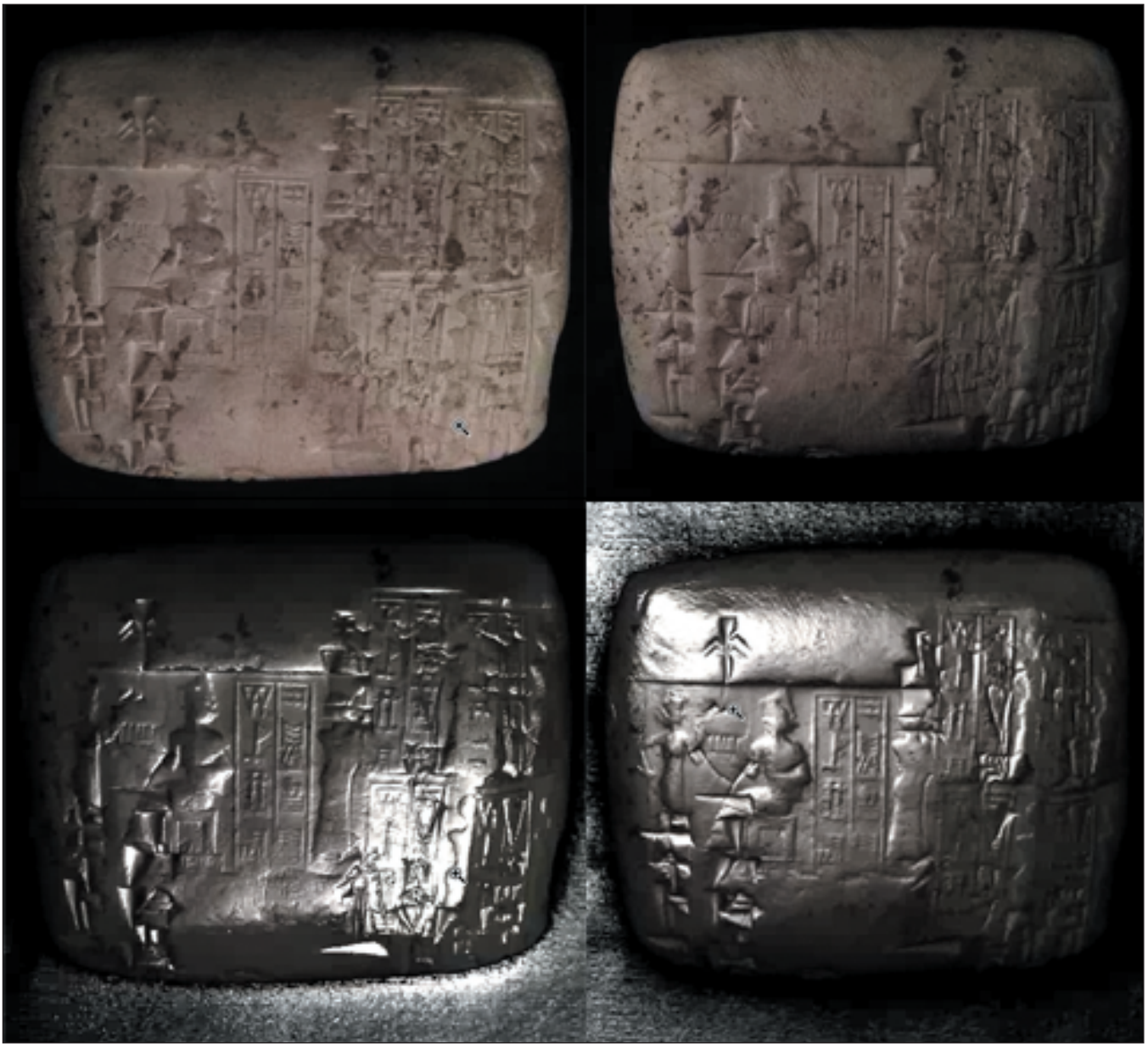
Figure 51. Images of an ancient clay tablet with different illumination positions (top), and rendered as a metallic surface to reveal subtle detail (bottom).
