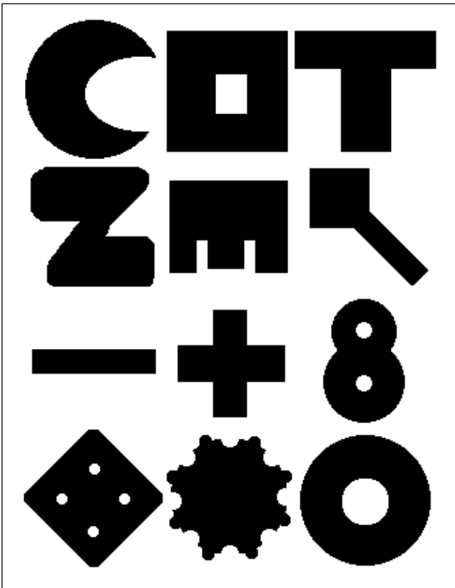
Figure 61. Twelve visually different shape with identical values of the shape parameter 4 \pi \text{ Area} / \text{Perimeter}^2
